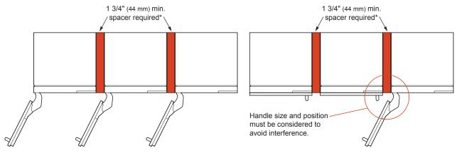
\*When using the Stainless Steel Door Panel Kit w/Handle or 3/4" (19 mm) custom panels with our optional Brushed Aluminum Handle, a minimum spacer of 1 3/4" (44 mm) between units is required to open each door 115° without interference.
