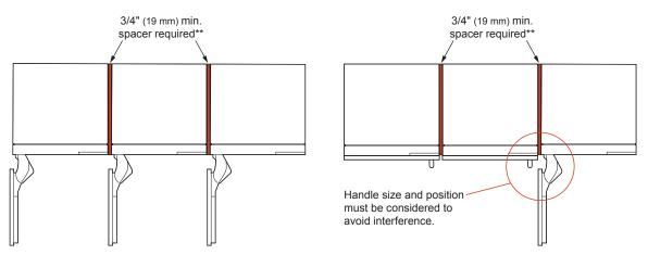
\*\*When using the Stainless Steel Door Panel Kit w/Handle or 3/4" (19 mm) custom panels with our optional Brushed Aluminum Handle, the door swing can be limited to 90°, reducing the minimum spacer between units to 5/8" (16 mm).
