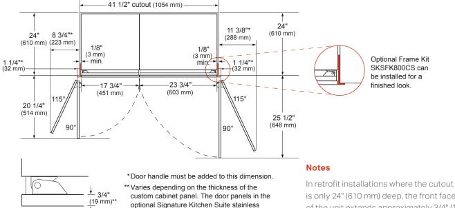
steel door panel kit are 3/4" (19 mm) thick.
