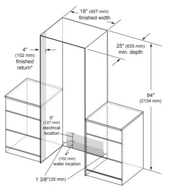
\*A minimum 4" (102 mm) finished return that matches the cabinet exterior is recommended on all sides and the top of the cutout opening. The shaded area will be visible after installation.
