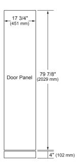
24-INCH INTEGRATED COLUMN REFRIGERATOR AND FREEZER
