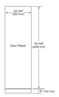
30-INCH INTEGRATED COLUMN REFRIGERATOR AND FREEZER
